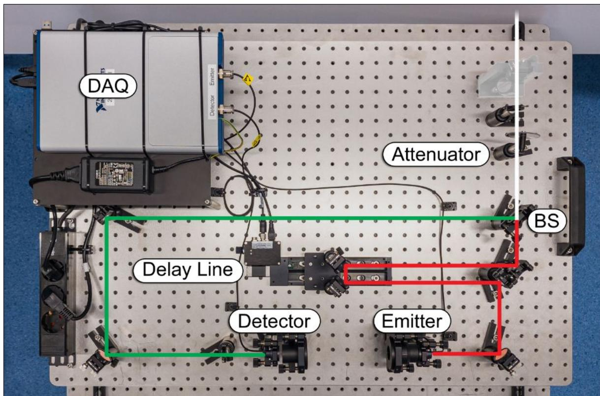
Figure 2: Designated laser beam path with free space antennas
