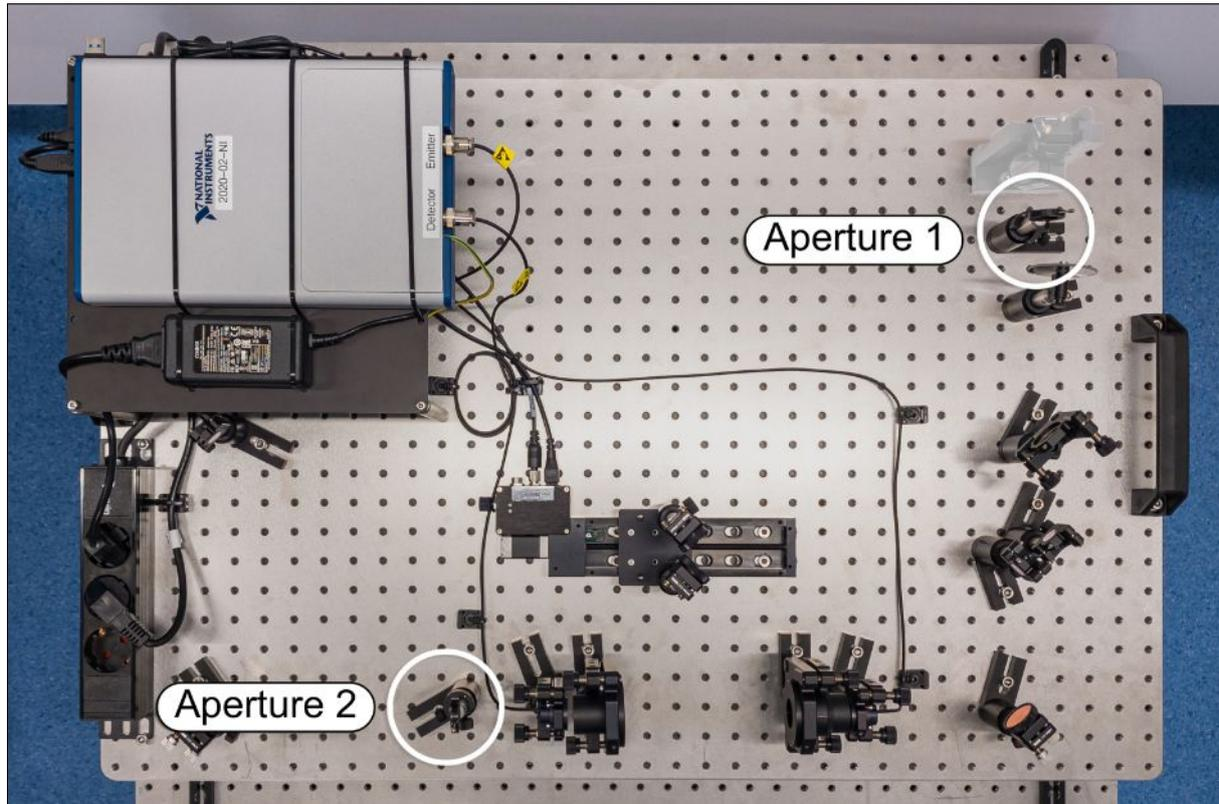
Figure 1: Apertures of the TDS10XX-wol for the alignment of the laser beam
