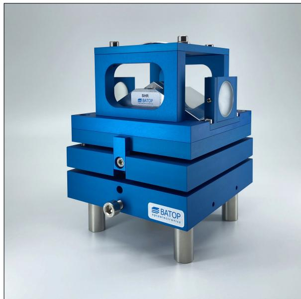
Figure 4: Sample Holder Reflection on the mandatory Sample Holder Base
