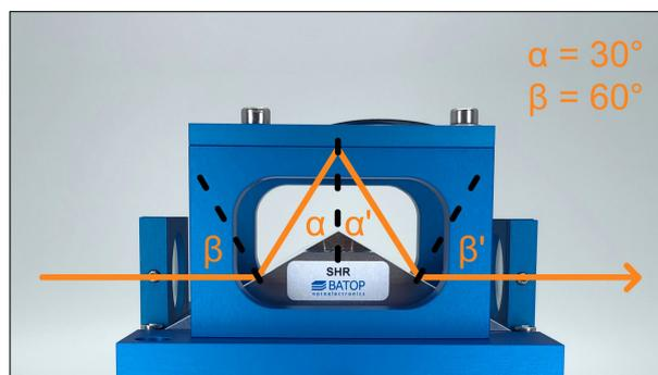
Figure 5: THz beam path in the Sample Holder Reflection
