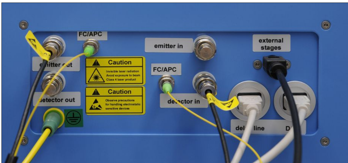
Figure 11: Orientation of the fiber connector to the fiber port
