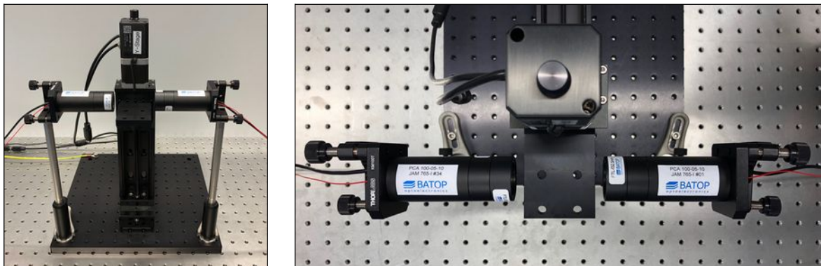
Figure 7: Imaging Unit set up for transmission measurements with a focused THz beam using our Extender Tube and focusing TPX lens ( FTL-f32.5mm )
