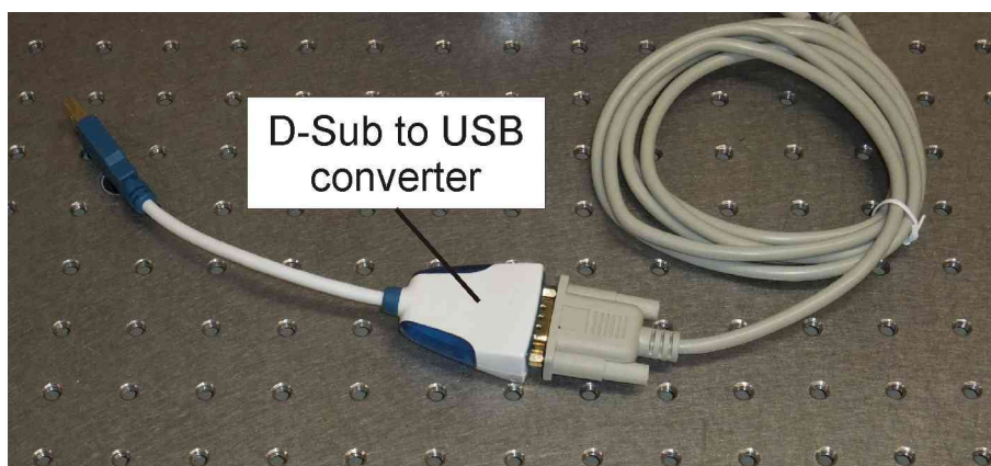
Figure 3: D-Sub to USB adapter for connecting the voice coil controller.
