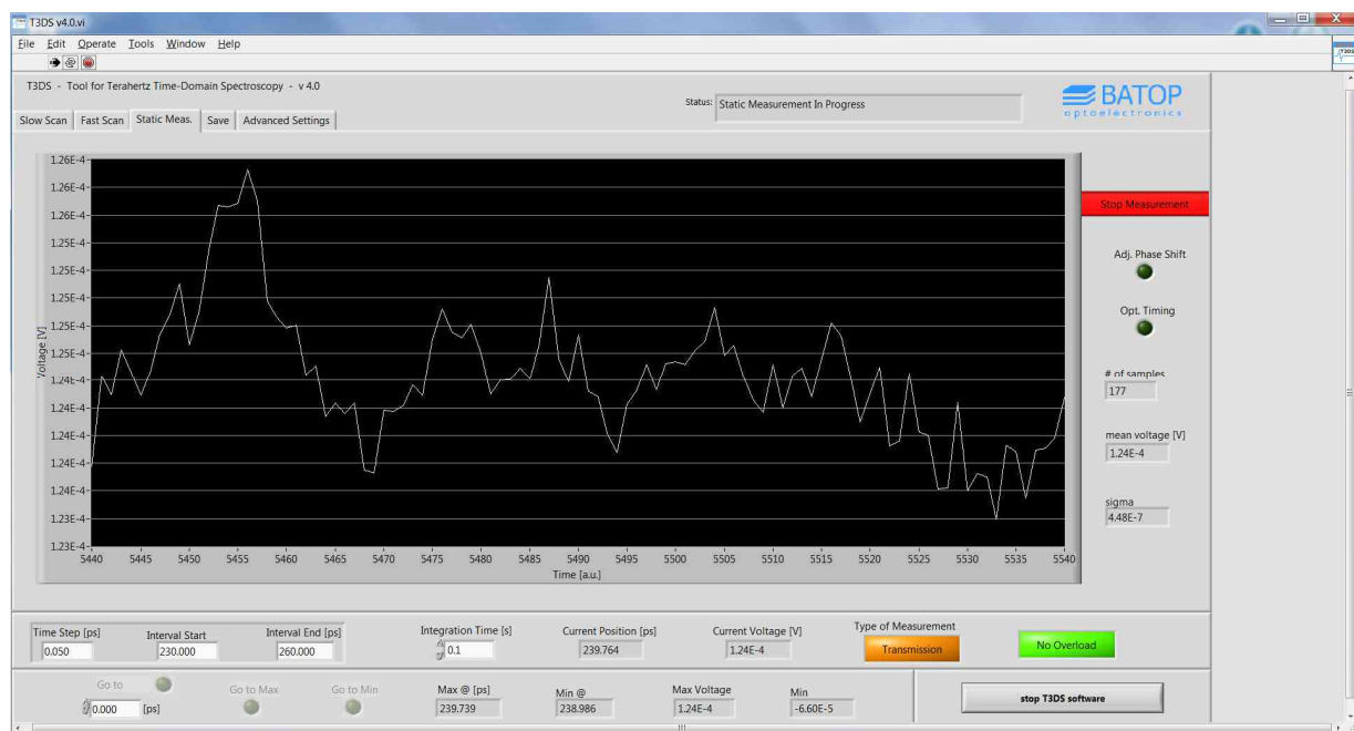
Figure 9: Static measurement mode showing the signal strength as a function of time after adjustment of the optical and terahertz path (T3DS v3.2).
