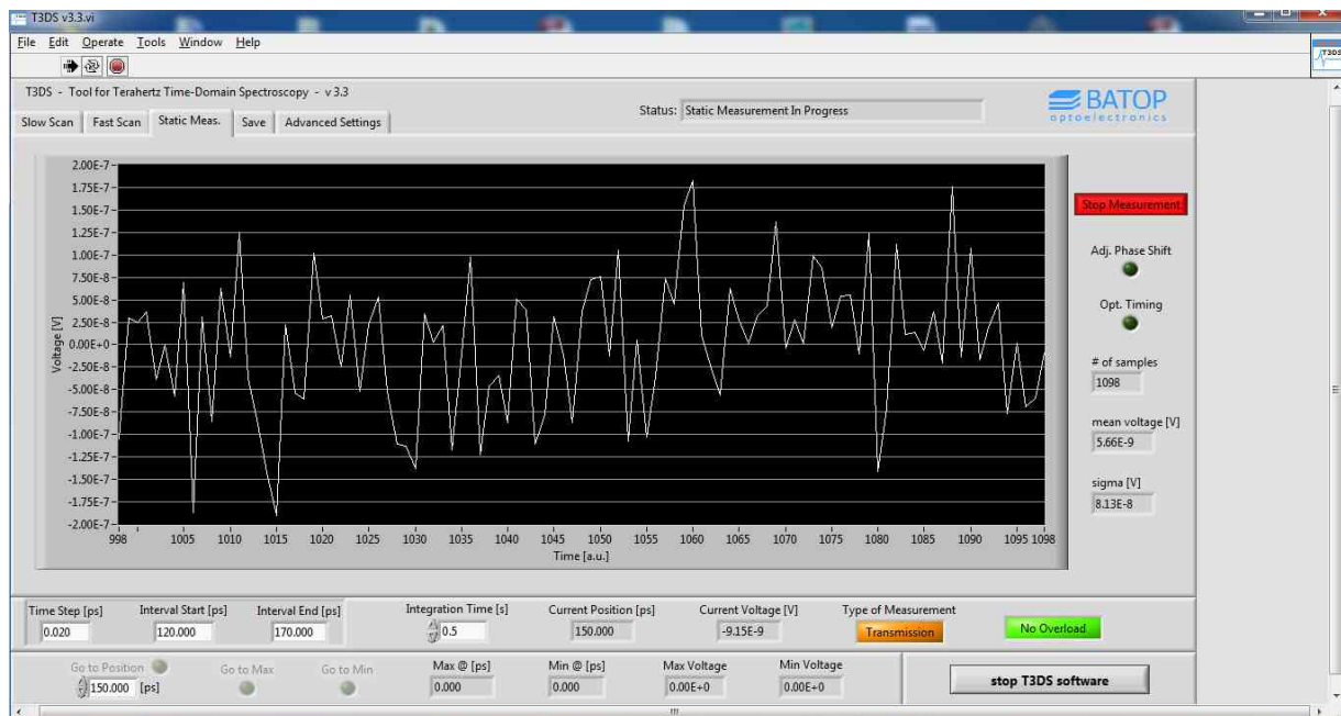
Figure 10: Static measurement to determine the noise voltage (sigma).
