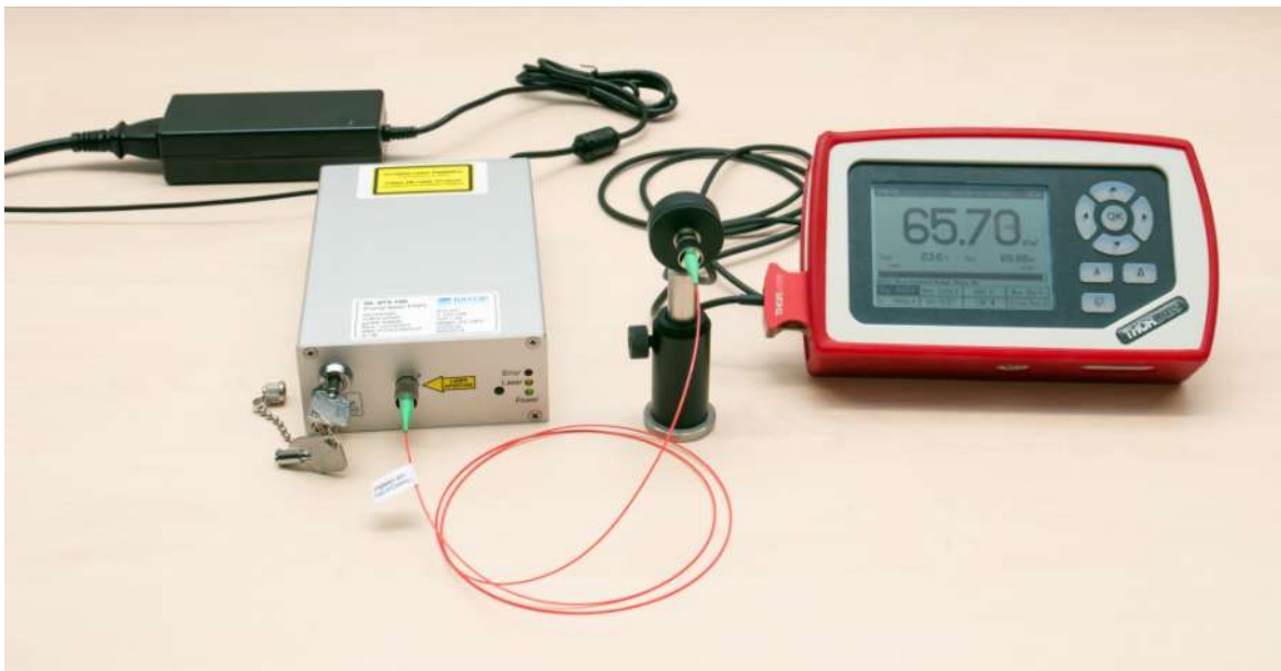
Figure 5.2.1 Setup for measurement of the diode laser DL-975 output power as a function of the drive current. The optical power meter is shown on the right side.
