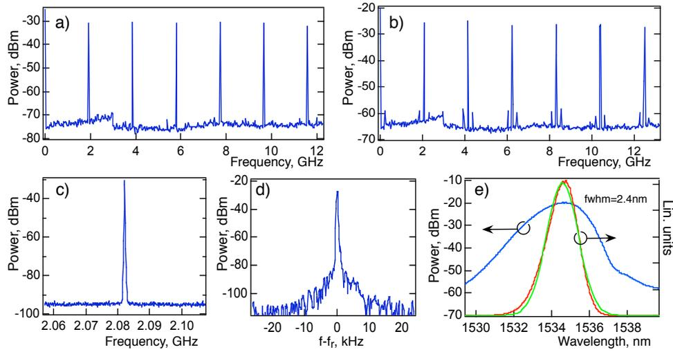
Fig. 3. Measurements of the Yb-Er fiber laser with  $f_r$  near 2 GHz (using the  $\Delta R = 0.11$  SAM). (a) Microwave spectrum with multiple harmonics of  $f_r$ . (b) Similar to (a), but showing sidebands that are a manifestation of slightly elliptically polarized light. (c) Field spectrum of  $f_r$  with a 50 MHz span and RBW = 100 kHz. (d)  $f_r$  at RBW = 300 Hz (e) Optical spectrum: the green trace is a Gaussian fit to the linear profile of the measured red trace beneath.
