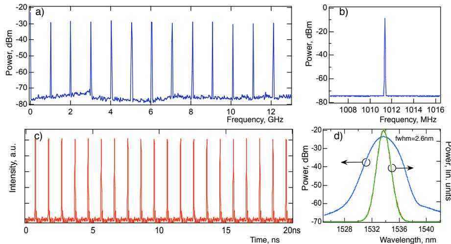
Fig. 2. Measurements of the 1.01 GHz Yb-Er fiber laser. (a) Microwave spectrum with multiple harmonics of  $f_r$ . (b) Field spectrum of  $f_r$  with a 10 MHz span and res. bandwidth = 10 kHz. (c) Pulse train (d) Optical spectrum: the green trace is a Gaussian fit to the linear profile of the measured red trace beneath, while blue trace shows the spectrum on a logarithmic scale.
