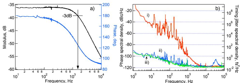
Fig. 4. (a) Response function of the MLL's output intensity with respect to the current modulation of the pump laser. (b) One-sided phase spectral densities of the  $2 \times f_r = 1.07$  GHz signal of a cw mode-locked Yb-Er laser. Trace (i), open loop; (ii), closed out-of-loop; and (iii), measurement system noise floor. The right axis shows the corresponding timing jitter spectral density.
