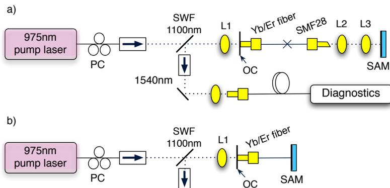
Fig. 1. Layout of two Yb-Er fiber lasers used in this work. They both form cw mode-locked lasers. SAM, (semiconductor) saturable absorber mirror; SWF, short wavelength pass filter; PC, polarization controller; OC, output coupler; L1 and L2, lenses with focal length = 11 mm; L3, lens with focal length = 4.5mm. Solid lines represent fiber, and dotted lines, air paths.
