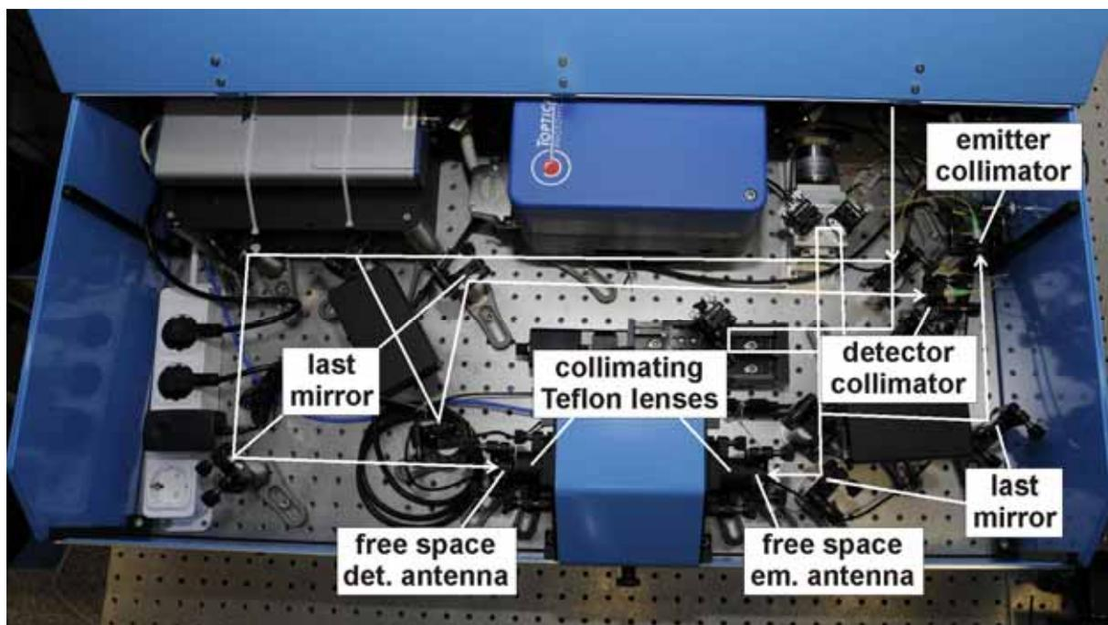
**Figure 3: Inside of a spectrometer with free space antennas and collimators for fiber-coupled antennas. Please use the last mirrors as well as the mounts with the free space antennas and collimators to optimize the antenna resistance for the free space / fiber-coupled antennas.**
