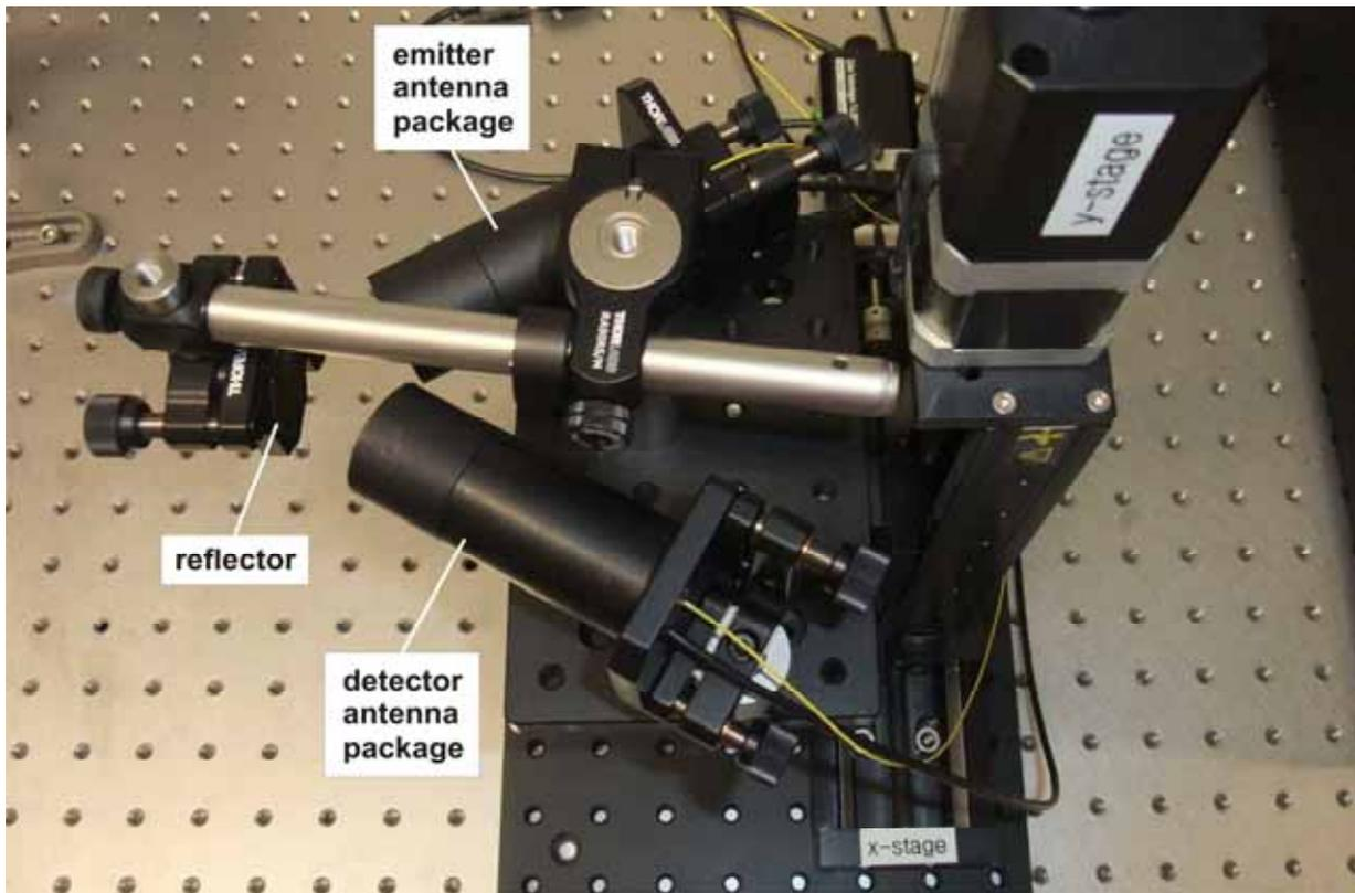
**Figure 7: Fiber-coupled THz antennas in a reflection setup for imaging purposes.**
