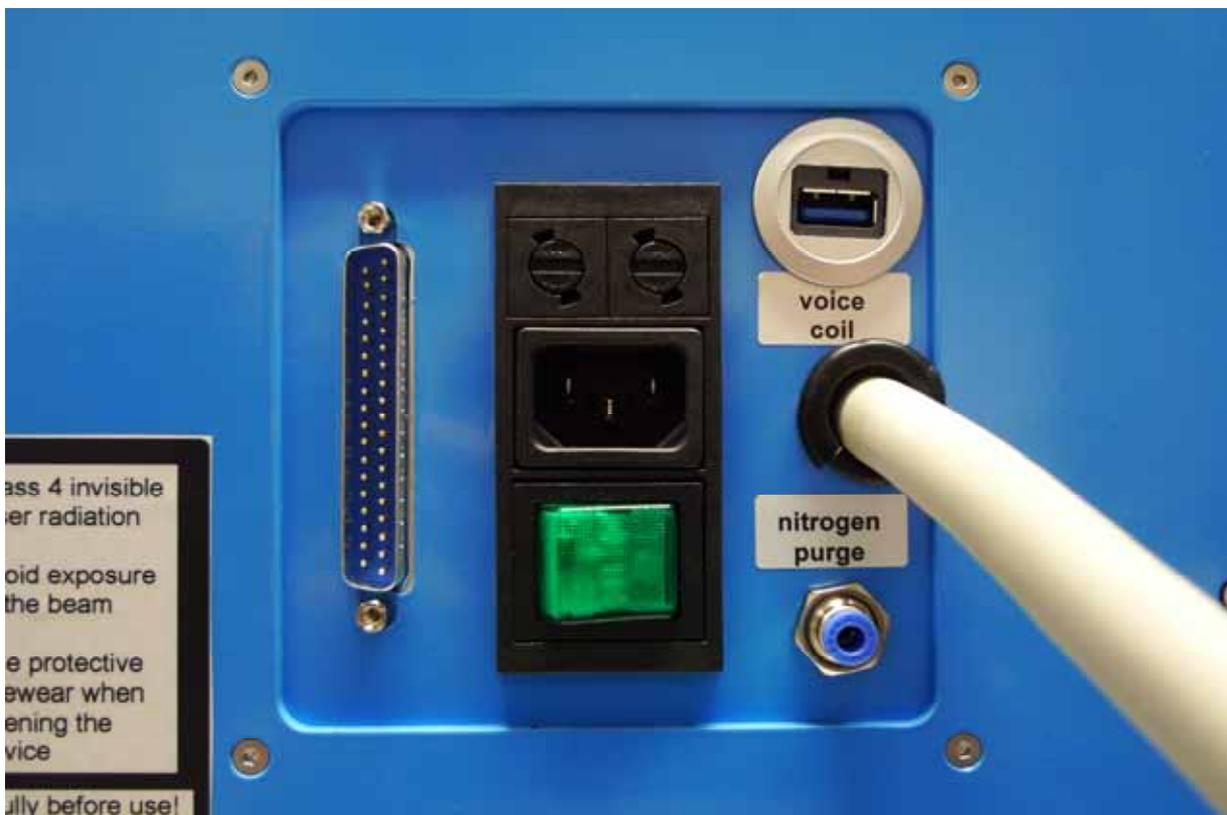
**Figure 1: Backside panel of a TDS system with power supply, nitrogen purge and the voice coil USB-connector which enables the fast scan option in the T3DS software.**
