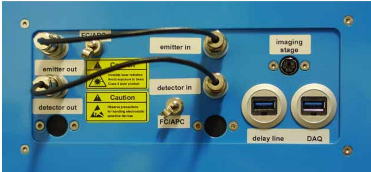
**Figure 2: Panel on the right hand side of a TDS system with ports for electrical and optical connection of internal / external antennas, the imaging stage, the delay line and the data acquisition system (DAQ).**
