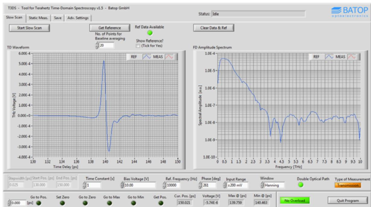
Figure 8: Result of a slow scan measurement displaying the time-domain and FFT data.
