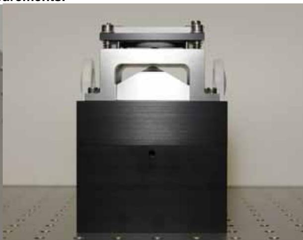
**Figure 6: Sample holder for reflection measurements.**
