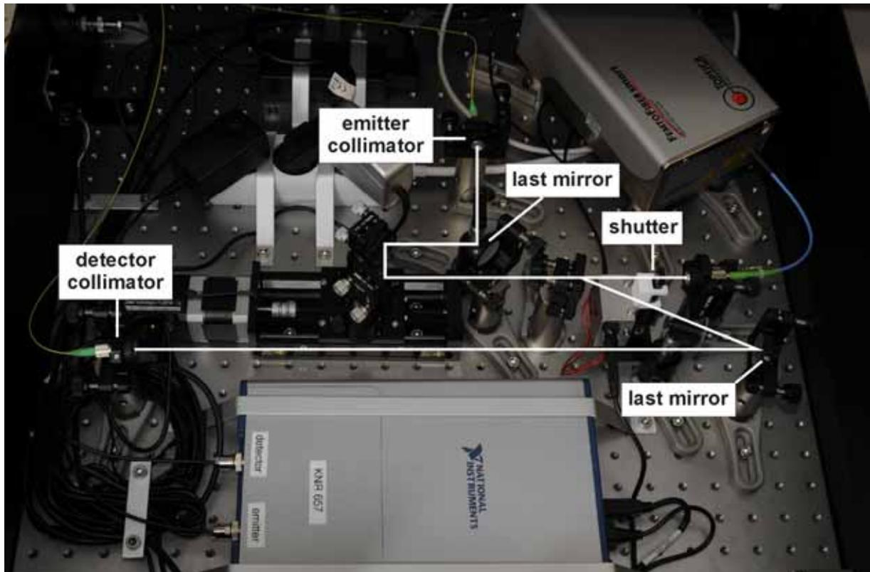
Figure 4: Inside of a fiber-coupled spectrometer. Please use the collimators and last mirrors before the collimators for optimizing the light coupling into the optical fibers.
